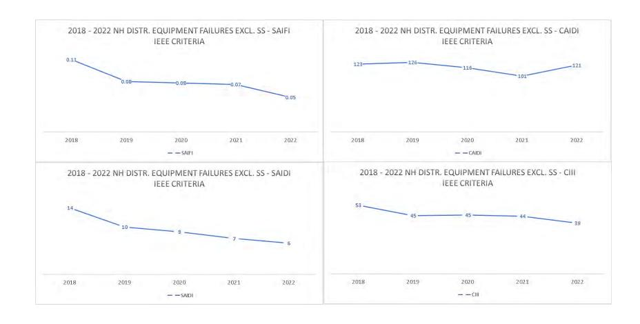
Section 1.5 SAIFI, SAIDI, CAIDI, CIII - Distribution Substation Equipment Failures - IEEE Criteria
